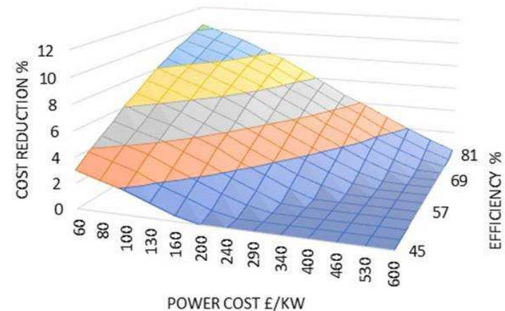
Percentage reduction in the cost of electricity with ACAES + H 2 storage compared to H 2 storage only
