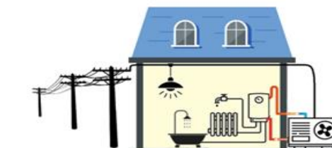
Provision of heating energy by air-source heat pump
